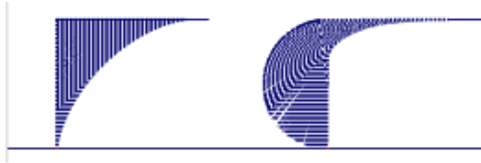
Drawing 2. Different types of sliding doors of a garage, viewed from the side.
